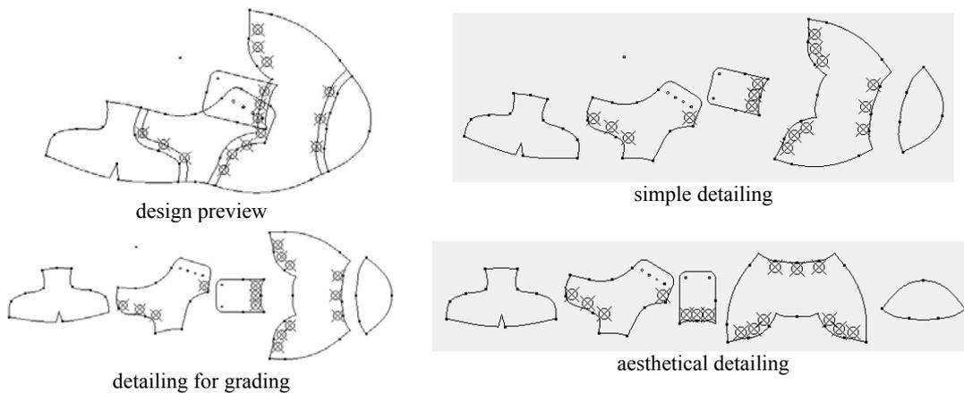
**Figure 8.** Footwear design by rendering – parts detailing (several layouts)
