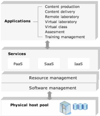
**Figure 2.** Hybrid cloud architecture
